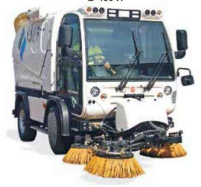
Reach up to 2800 mm hopper, Capacity 4m3
