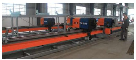
$\succ$  The metal bender also has an excellent adaptability.It can process III class rebar of  $\phi$ 10-32(HRB400).
